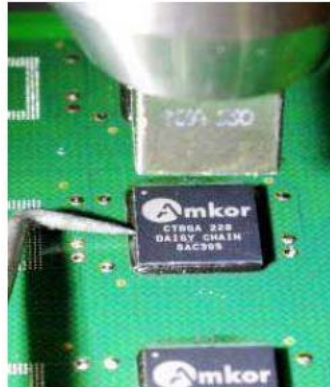
Figure 9-7: Removing Underfill Using Steel Probe
