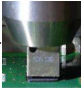
Figure 9-6: SRT Nozzle Lowered 2 mm to 3 mm from Component Top Surface
